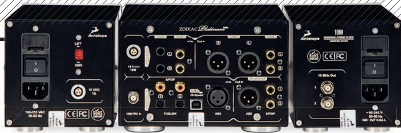
ABOVE: The DAC [centre] offers USB (with a 10MHz clock input on BNC), coaxial and Toslink S/PDIF, and AES/EBU digital ins, re-clocked S/PDIF and AES digital outs plus RCA and balanced XLR analogue outs. The 10M [right] provides two clock outputs
